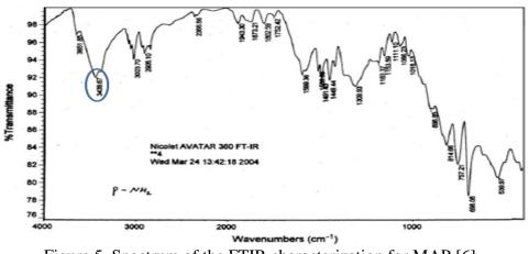
Figure 5. Spectrum of the FTIR characterization for MAP [6].
