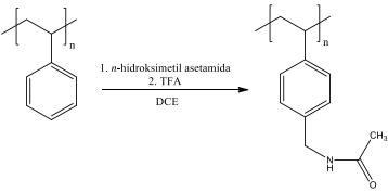
Figure 2. The formation reaction of AMP [2].
